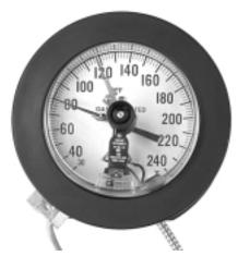
The electric contact feature is a switching mechanism actuated by the indicating pointer Switch points are adjustable and can be set throughout the 270° arc. Contacts are used to activate alarms and relays.
