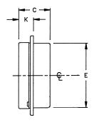
Front flanged case for semi-flush mounting.
