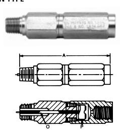
**Piston Type:** Shocks and pulsations are absorbed in the doughnut-shaped orifice (0) formed by the piston (P) in the tube. As the piston moves up and down with the pulsation, it automatically clears away any sediment or pipe scale that would clog a simple orifice or needle valve.
